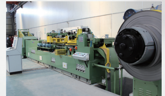
硅钢片（数控）横剪生产线 Step lap cut-to-length line for transformer CRGO lamination
